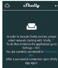
Press the home button of your iPhone/iPad/iPod. Open Settings > WiFi and connect to the WiFi network created by Shelly, e.g. shelly1pm-35FA58. If using Android your phone/tablet will automatically scan and include all new Shelly Devices in the WiFi network that you are connected to.
